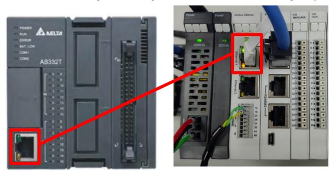
II. The gateway's first 485 port is connected to the interface module 0170-0101 before being connected to the control module via an Ethernet cable
